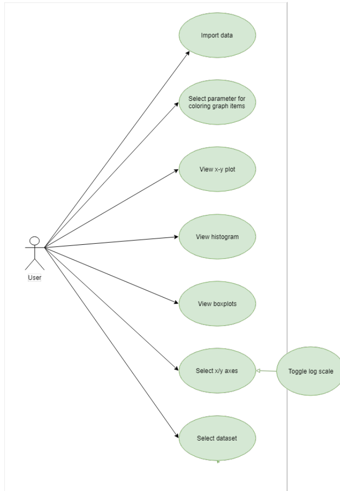
Figure 4.6: Use cases related to statistical graphs include importing data, selecting parameter for coloring data, displaying four types of graphs, toggling between linear/logarithmic scales and selecting dataset
