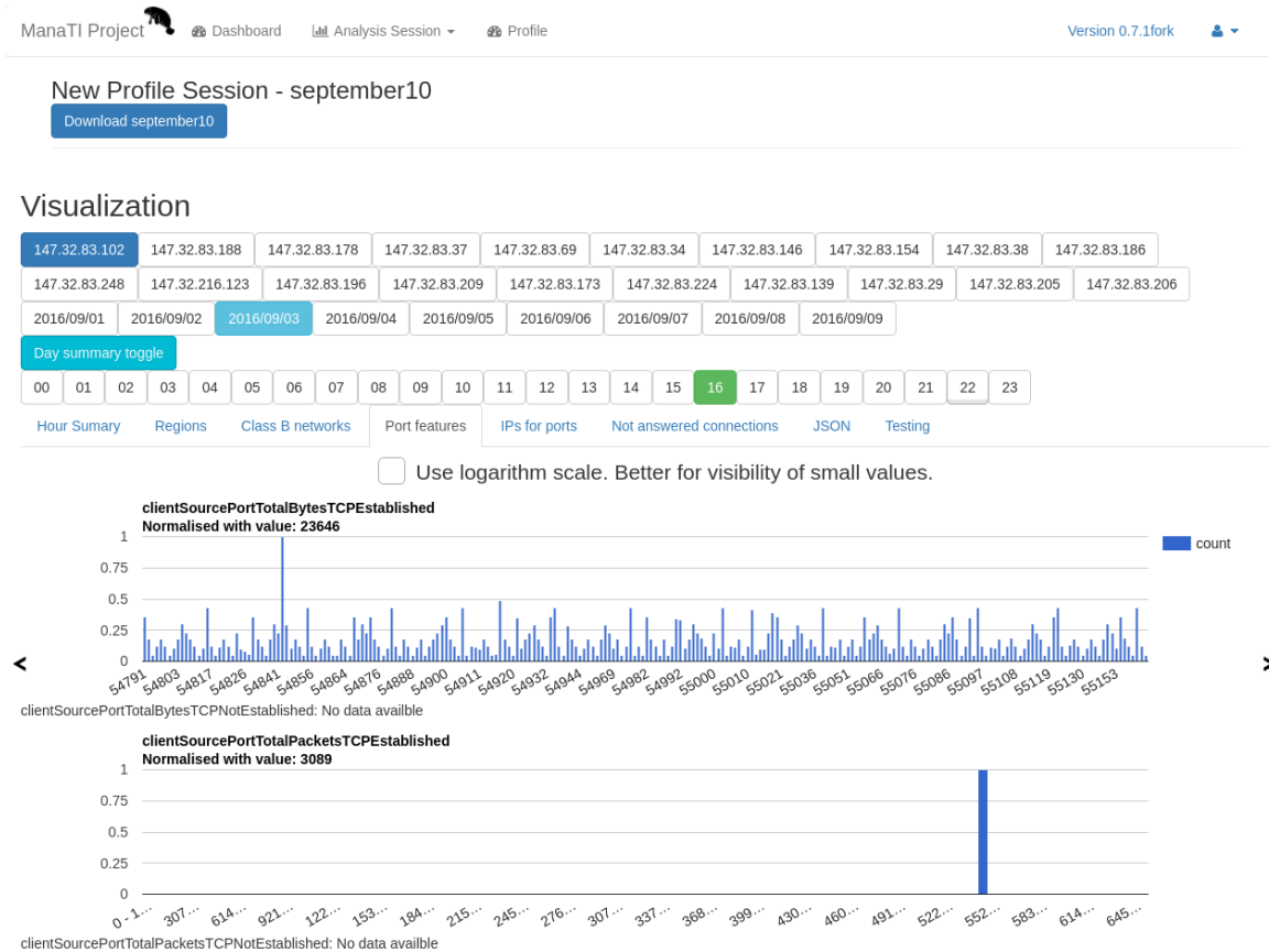
Figure 3.5: Port features. Two features are visible in the screen-shot. In this case features "clientSourcePortTotalBytesTCPEstablished" and "clientSourcePortTotalPacket-sTCPEstablished". The second graph show histogram of ports and the first graph shows one of the bins expanded.
