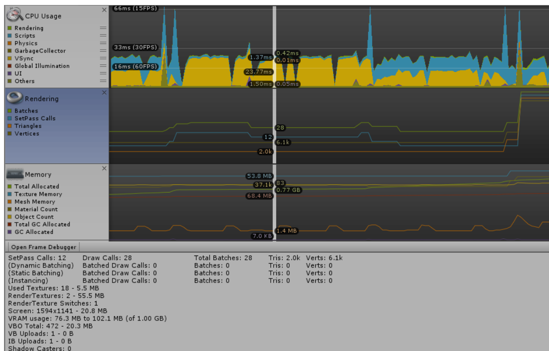
Figure 5.1. Performance testing using Unity Profiler
