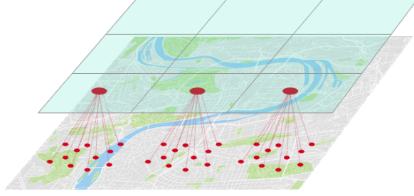
Figure 5.2: Example of collecting graph's elements in each cell of the distribution grid.
