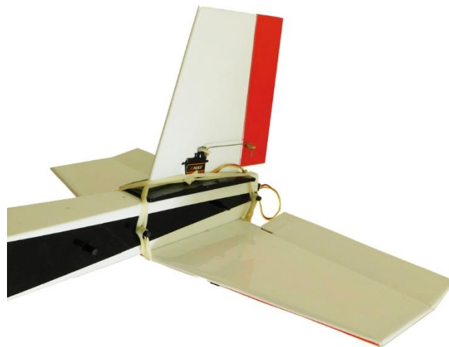
Figure 9: Tailplane Mount and Rudder Servo Placement
