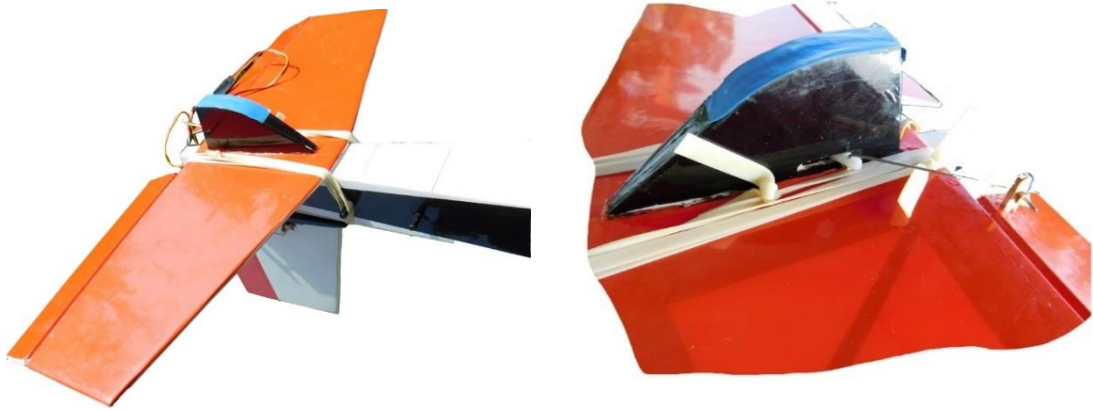
Figure 10: Horizontal Stabilizer Mount to the Bottom of Rear Fuselage and Elevator Servo Mount
