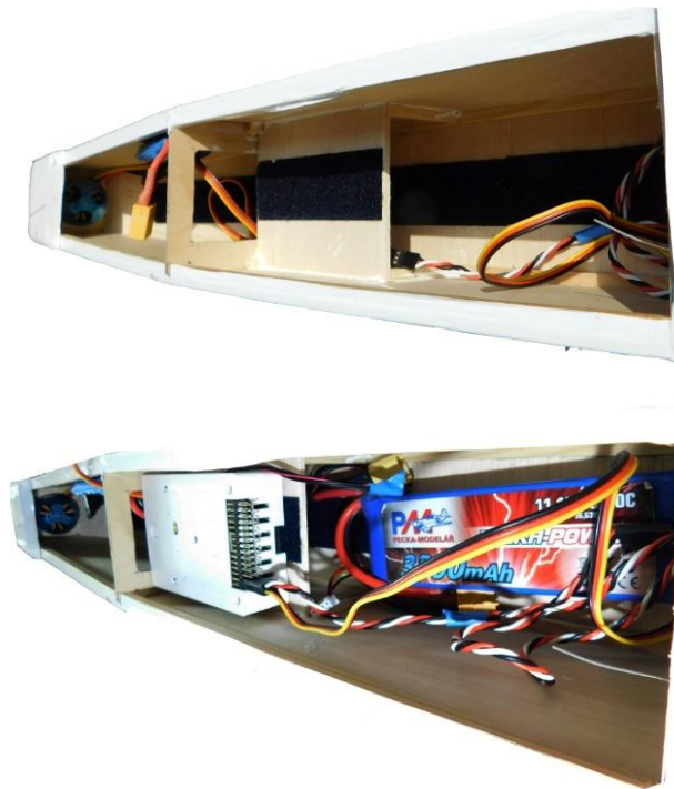
Figure 12: Spacious Fuselage with Velcro stripes and component placement
