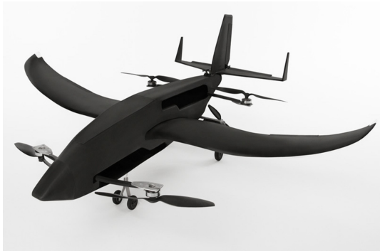
(a) Example of VTOL UAV. Credits: The Register 1
