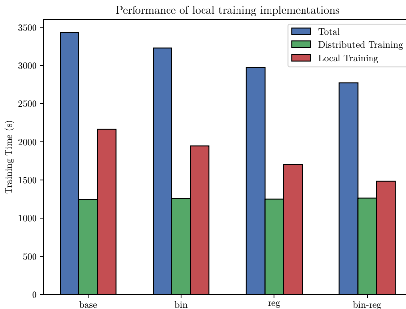
Figure 5.3: Comparison of multiple-tree local training scheduling methods for 5 trees with 30M data
