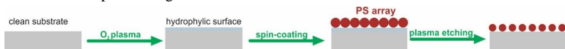
Figure 5.1 A schematic drawing of the steps involved in the mask preparation and modification.
