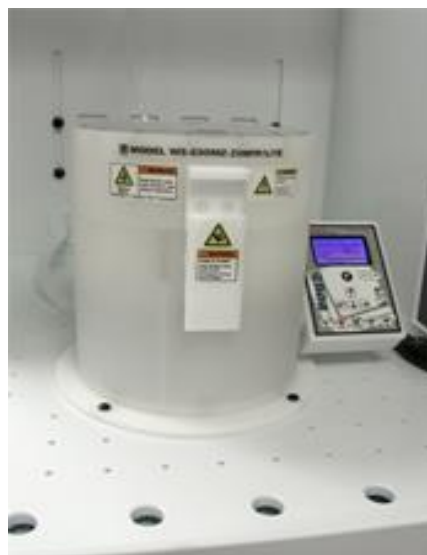
Figure 4.4 Spin-coating instrument (WS-650Sz Lite Single Wafer Spin coater) [199].
