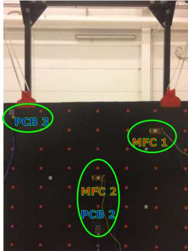
Figure 5.2: The test article: a composite plate bonded with MFC piezo actuators and PCB accelerometers.
