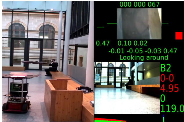
Figure 5: UAV-UGV team performing autonomous inspection. The ground robot is guided by the navigation system described. See a video at https://youtu.be/RPCUB6xjQTI
