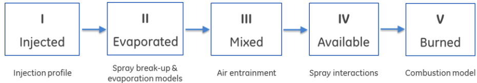
Figure 37 Diesel spray combustion model structure describing fuel transformation path
