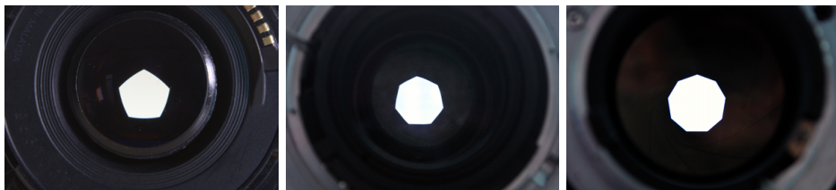
(a) The pentagonal aperture. (b) The heptagonal aperture. (c) The nonagonal aperture.
