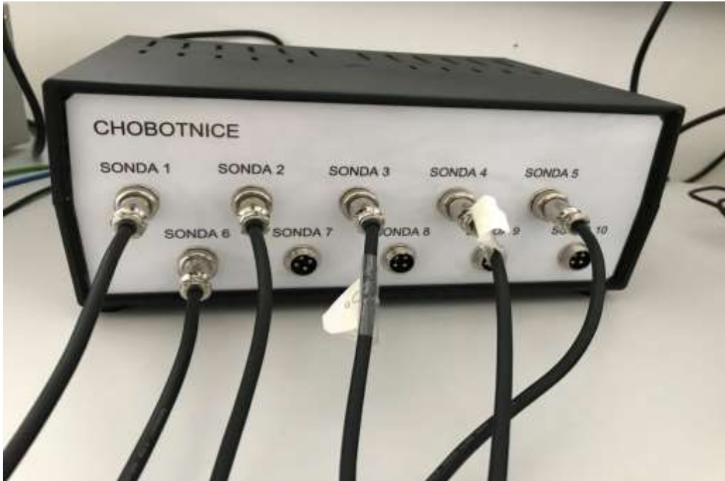
Figure 6: 'Chobotnice', device to measure pressure at 10 inputs
