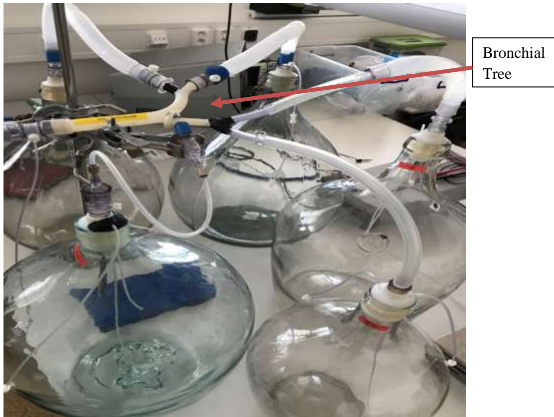
Figure 4: Demijohns representing compartments of the lungs
