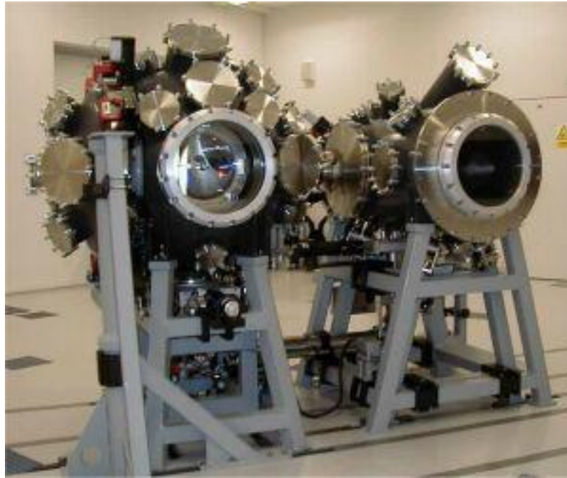
Figure 17: Master (on the left) and secondary (on the right) interaction chamber at PALS [42]
