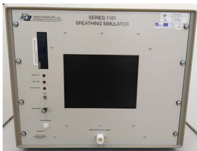
Obr. 1.5: Aktivní model plic Series 1101 Breathing Simulator (Hans Rudolph, inc., Shawnee, Kansas, USA).
