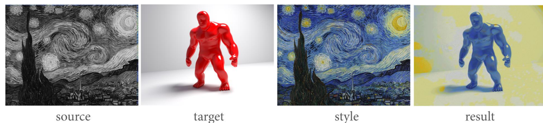
Figure 5.15: As the target guiding channel I used only the RGB image of the Golem render. I created my own source channel by using a grey-scale version of the painting. Note that the histogram of the source channel can affect the overall result and gives a lot of space for customisation. The synthesis with those two channels, however, does not transfer the artistic style, only colours.
