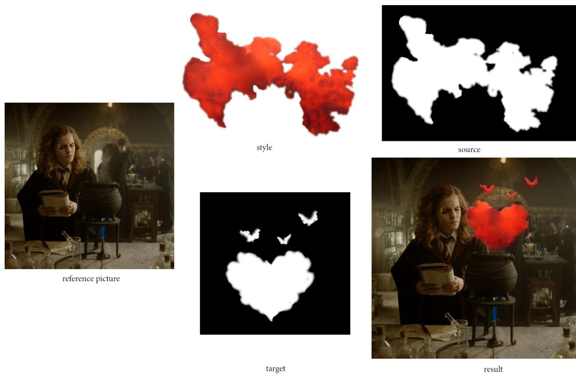
Figure 5.34: Example of cloud synthesis using two alpha images as source and target guiding channels.
