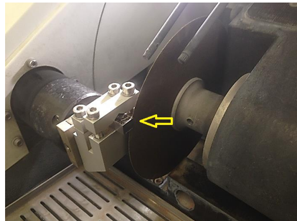
Figure 18: cutting of the sample
