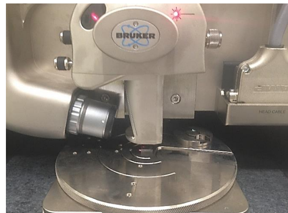
Figure 28: Sample mounted on the AFM table
