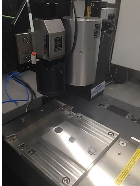
Figure 26: Sample mounted on the magnetic table of the nanoindenter
