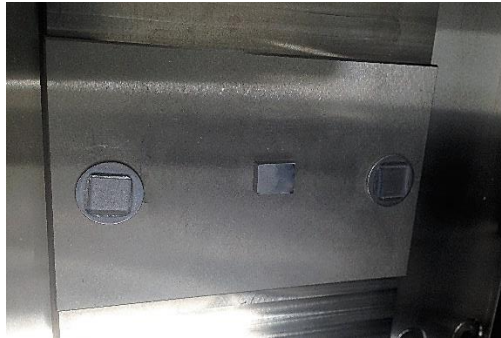
Figure 31: Magnetic table for sample mounting during room temperature nanoindentation
