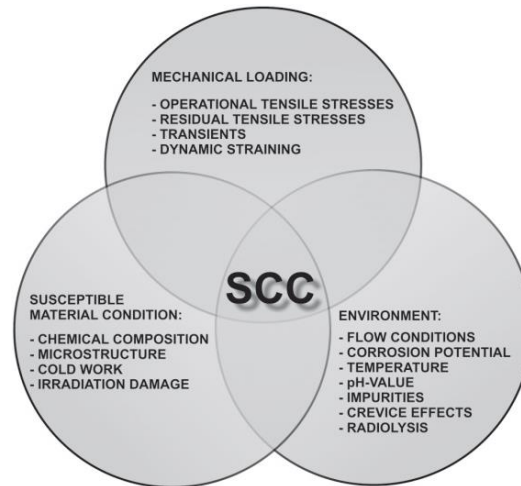
Figure 8: Scheme of SCC conditions – source: Stress Corrosion Cracking in Light Water Reactors :Good Practices and Lessons Learned, 2011, pg. 4
