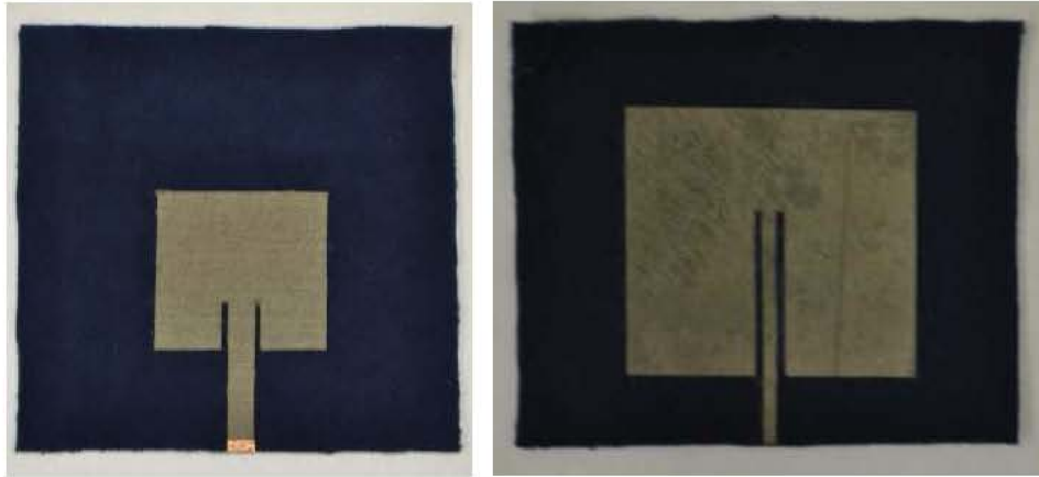
Fig. 54 Betex microstrip patch (left) and Cu/Ni microstrip patch (right).
