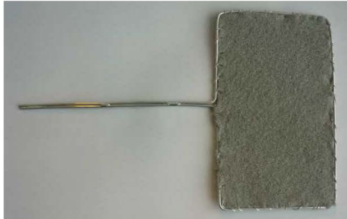
Fig. 36 Sample of PP textile – vacuum deposition of tin.
