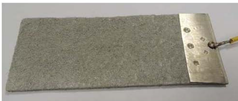
Fig. 37 Monometallic tin felt electrode ready for filling (non-woven PP textile carrier prepared by needling).
