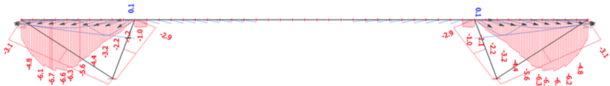
FIGURE 134: FIRST TENSION VALUES 70 METER BEAM-3 TENDONS
