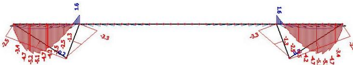
FIGURE 121: TRIANGULAR FRAME TOP STRESSES FORTH ITERATION.
