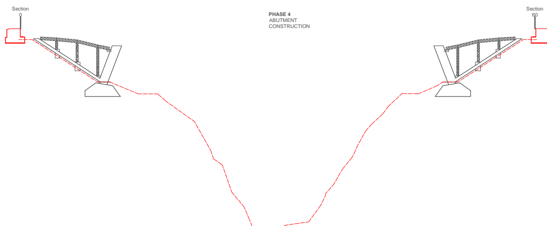
FIGURE 181: CONSTRUCTION STAGES STAGE 4
