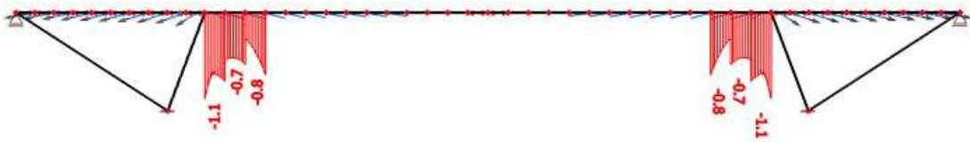
FIGURE 171: LAMELLA 3 BOTTOM FIBERS, FORMWORK CONSIDERED-OVERSTRESS STRUCTURE.
