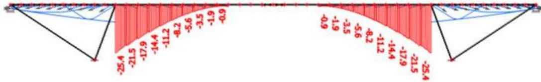
FIGURE 164: LAMELLA 10 BOTTOM FIBERS, FORMWORK CONSIDERED
