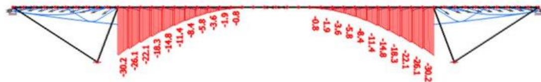
FIGURE 165: LAMELLA 11 BOTTOM FIBERS, FORMWORK CONSIDERED
