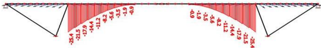
FIGURE 158: LAMELLA 10 BOTTOM FIBERS, FORMWORK CONSIDERED
