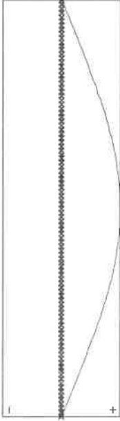
Figure 9 : Lateral displacement component of the shear centre (Mode 1)
