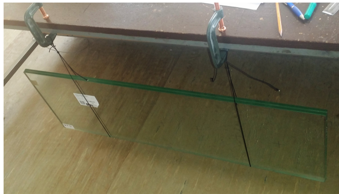
FIGURE 7.1: Experimental setup for simulation of free-free boundary conditions
