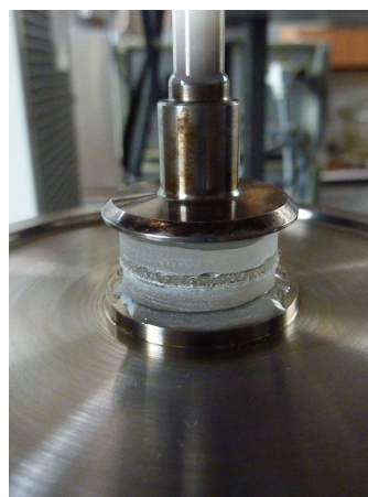
(B) Laminated glass specimen in rheometer
