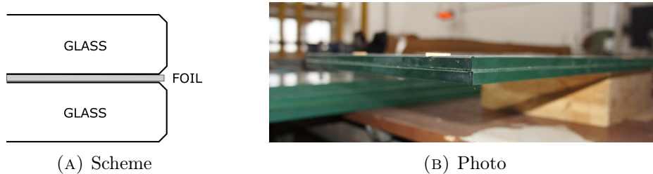
FIGURE 1.4: Three-layer laminated glass
