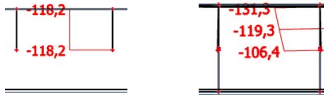
Picture 4.7-6 - average stress, linear behaviour (left) and stress diagram for non-linear behaviour (right)
