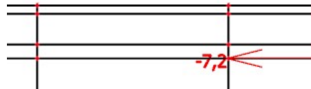
Picture 4.9-8 - long. deformation caused by deflection from traffic load (side with expansion bearing)
