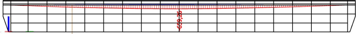
Picture 4.4-18 – maximal normal force caused by traffic load in longitudinal stiffener, midspan
