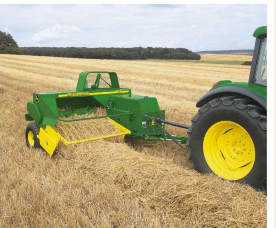
Crop control – and better bales – start here; with the low profile, high capacity pick-up, crop lift and leaf loss are minimised, thanks to the small diameter pick-up.
