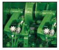
Needles, made of formed steel for long life, bring twine to the knotters after each cycle of the measuring wheel. And surgical quality steel twine knives are easily removed for sharpening or replacment.
