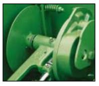
The needle brake facings maintain a constant force to keep the needle out of the balecase after the tying cycle, even in the roughest terrain, and prevent backslap. The brake is designed for durability and a long service life.
