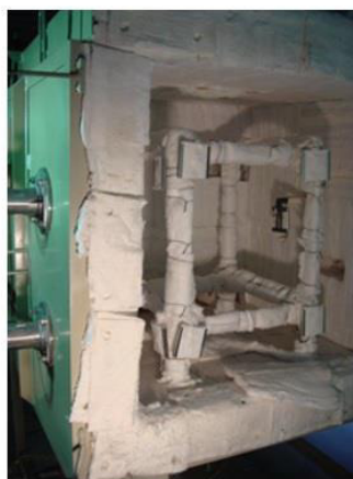
b) Geometric position for plate thermocouples inside furnace.
