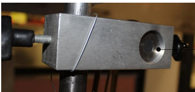
obr. 28: Detail instalace radiometru
