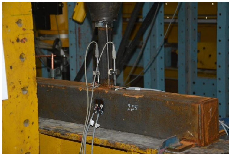
Figure 11 Strain gauge placement
