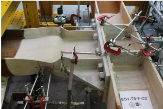
Figure 27 Failure mode on full-strength connection. Pictures by the Università degli Studi di Napoli Federico II, 2015.
