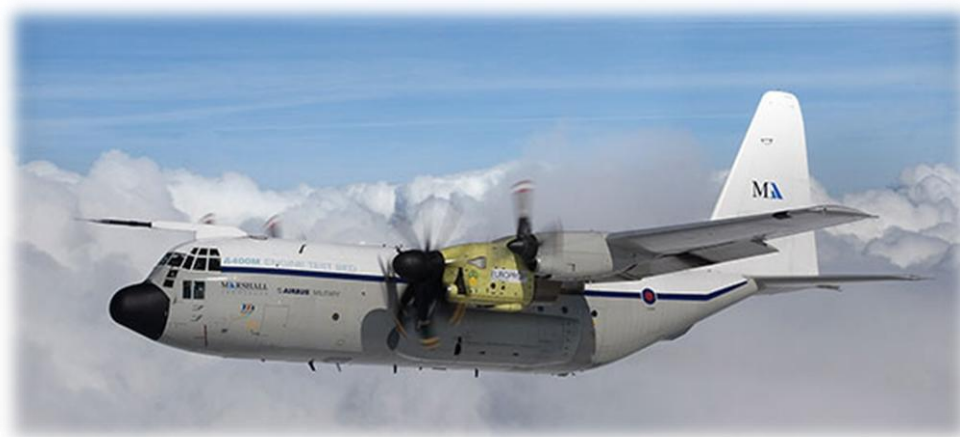
Obrázek 7: C-130 Hercules s testovaným motorem. (Zdroj: A400M Engine Flying Test Bed. In: Marshall Aerospace [online]. Cambridge, UK, 2017 [cit. 2017-05-10]. Dostupné z: http://marshalladg.com/a400m-engine-flying-test-bed/ )
