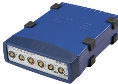
Figure 5.9: ETAS ECU interface unit. The hardware interface used to flash the test vehicle target with the compiled control software.
