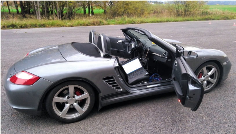
Figure 4.1: The test vehicle for torque vectoring. Flashing new version of the electric vehicle control system into the test vehicle on a closed airfield.
