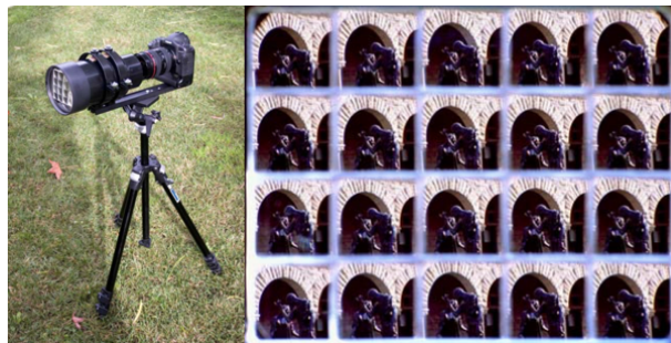
Figure 4.2: Second prototype of Adobe's light field camera (left) and set of 20 images obtained by this camera [21].
