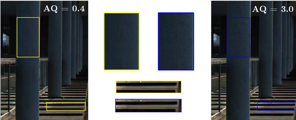
Figure A.2: Example of flat and detailed areas after processing with x264 with different AQ strength. Left - AQ = 0.4, right - AQ = 3.
