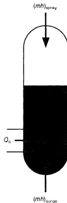
Figure 20 - One-region pressurizer - supplied mass flow rate, enthalpy and heat [13]
