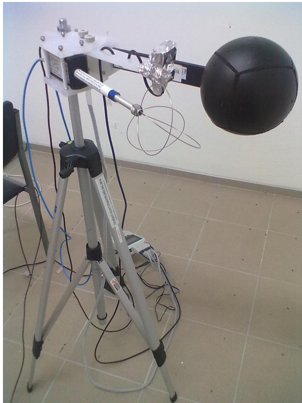
FIGURE 2. A globe stereothermometer and sensors for measuring the dry temperature and air velocity.
