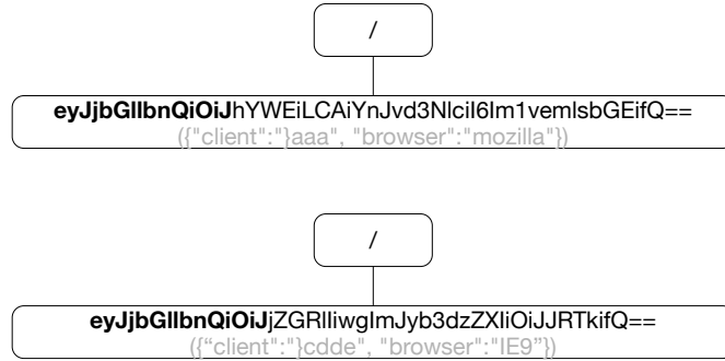
Figure 6.3: One of the options to tunnel data from client to server is to send base64 encoded json files. Figure shows an example of the path and data being sent.
