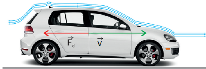
Figure 4.5. Drag between the fluid and the vehicle in motion [40]
