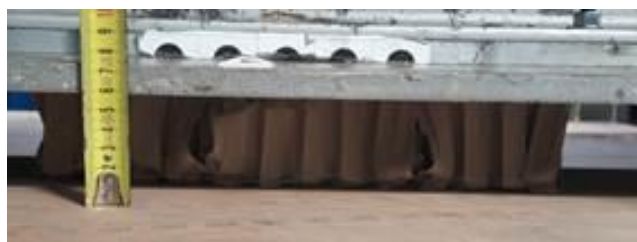
Figure 20: Calculation of the crushing of the carton
