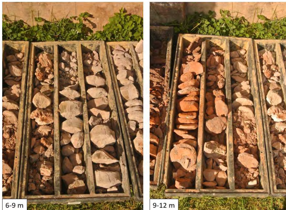
Figure A.4. Extracted soil tube from borehole beside the southern wall at depth 6-9m (left) and 9-12m (right)
