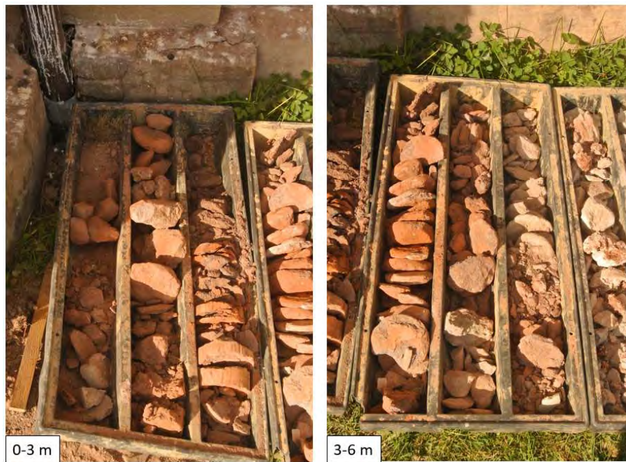
Figure A.3. Extracted soil tube from borehole beside the southern wall at depth 0-3m (left) and 3-6m (right)
