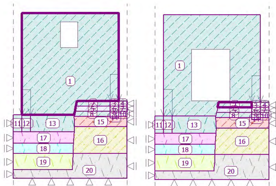
Figure 5.6. Modelling eastern (left) and western (right) transverse facade to analyse the stresses due to differential settlement
