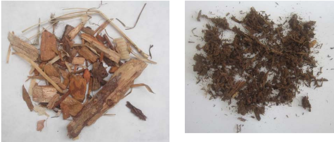
Fig.2.14 Untreated wooden chips on the left, treated (200° C) on the right [31].
