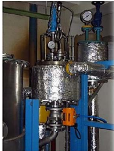
Fig. 2.12 Unit for thermal-expansive pretreatment TEP [31].
