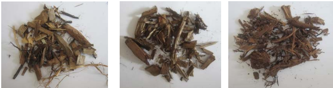
Fig 2.15 Treated wooden chips at different Temperatures (135° 160° 180° C) [31].
