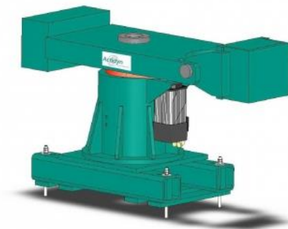
Figure 1-1 C60, geotechnical centrifuge [1]
