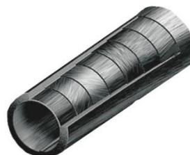
Obrázek 33: Vrstvy karbonové trubky ( http://www.better-digital-photo-tips.com/images/benro-monopod-leg-8-layer-carbon-fiber-composition.jpg )
