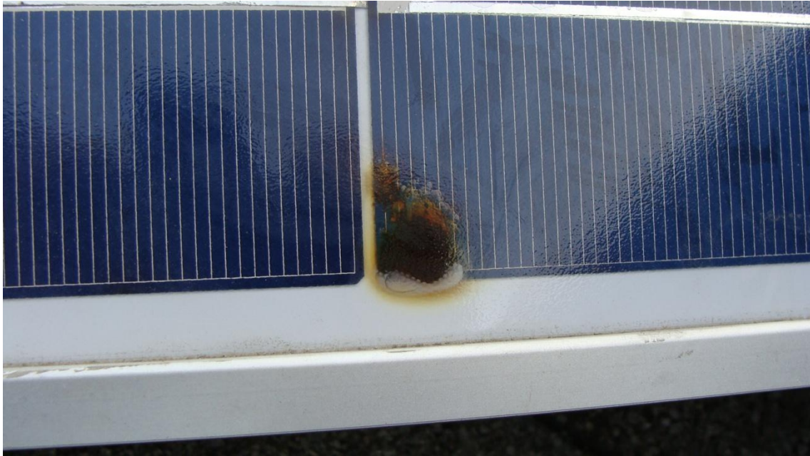
Fig. 26: Example of hot-spot
