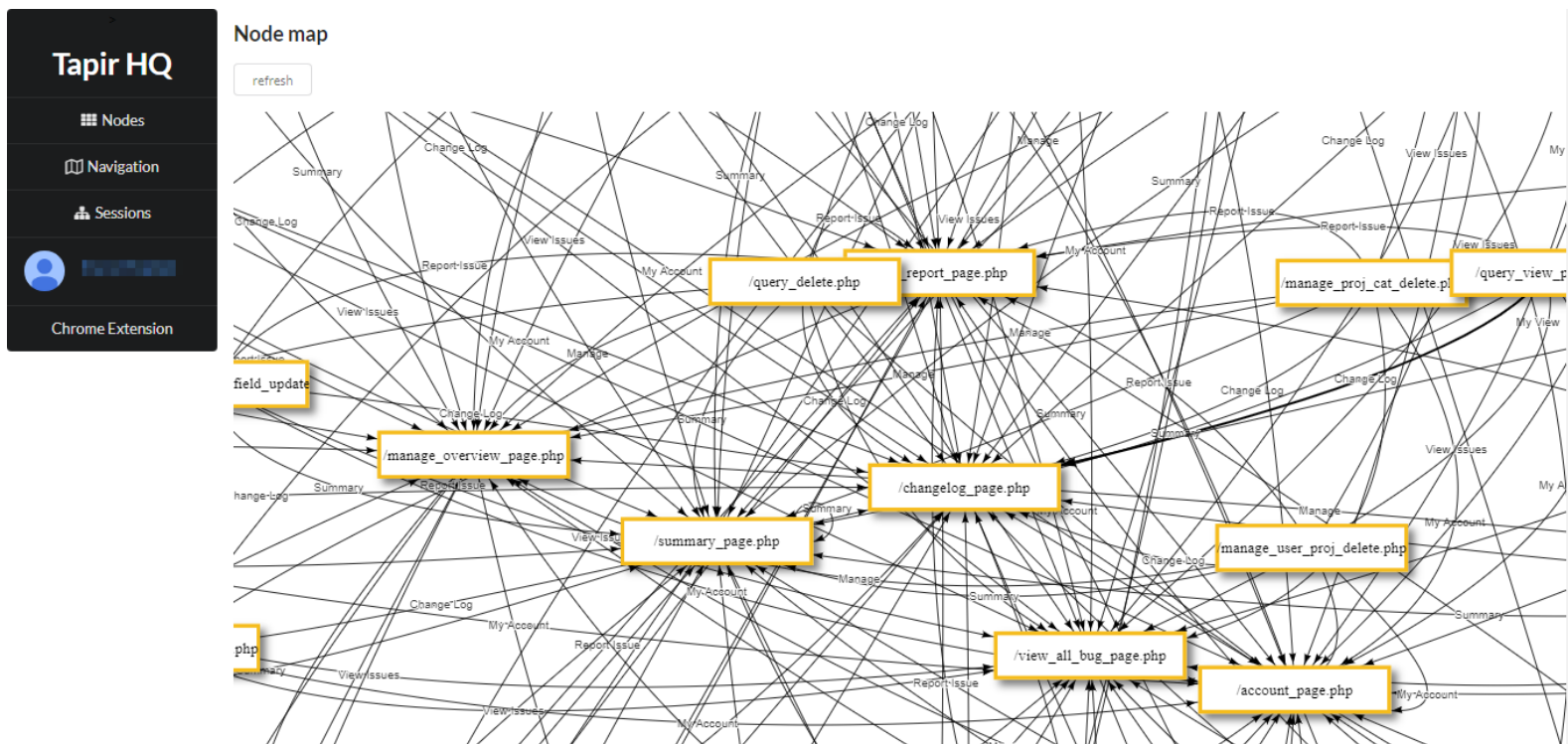
Figure 3.11: A sample from the Tapir Analytics module – SUT pages and possible transitions between them
