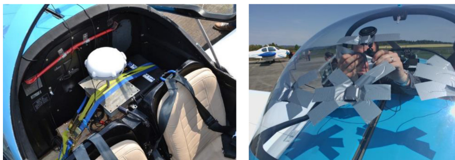
Fig. 7. Measurement assembly onboard aircraft Slingsby T67C in a sensory compartment with a referential GNSS system on the top (left) and GNSS antennae mounted on the cabin cover (right).
