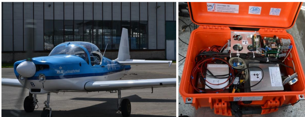
Fig. 6. Slingsby T67C aircraft (left), the sensory compartment inside Pelicase 1450 (right). (For interpretation of figures in color, the reader is referred to the web version of this article.)
