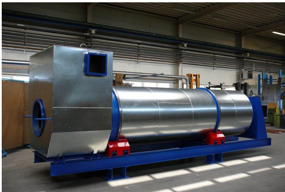
Figure 4.1 Steam drum dryer [13]
