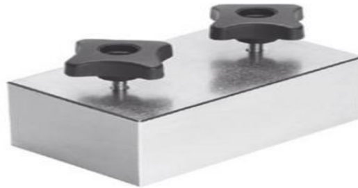
Fig. 29: Loading weight, 2 kg [8]
