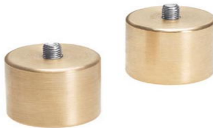
Fig. 30: Brass Loading weight, 0.175 kg [8]
