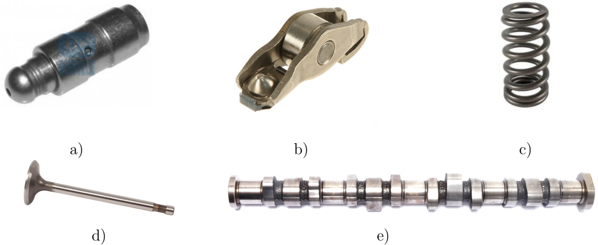
Figure 4.4: Real parts: a) Hydraulic lash adjuster, b) Rocker arm, c) Spring, d) Valve, e) Camshaft. 1
