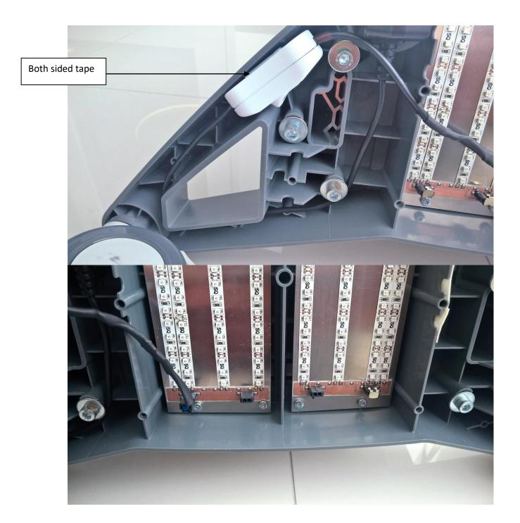
5. Connect both sheets using "Cable A" and twist it according to picture
