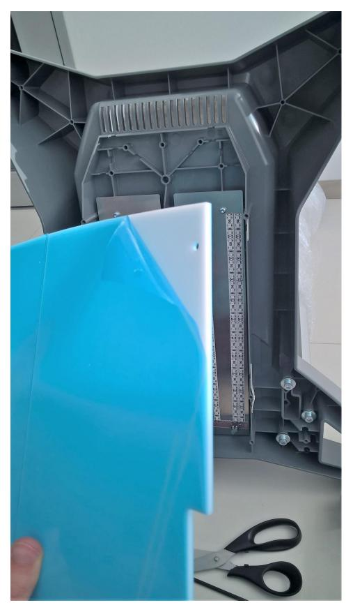
7. Install the Plexiglas cover using *4 screws A*. Gently push on the cover so that it rests nicely and doesn't have gaps around the adapter area
