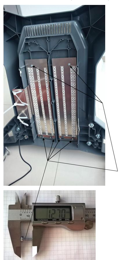
4. Connect the wire from adapter to the sheet socket. Adapter is movable in its holder so you can adjust the cable length so that the switch can comfortably be placed in place according to the picture. Remove foil from adhesive tape to glue it to the machine. Tighten strapping tapes and remove those, which aren't holding adapter.
