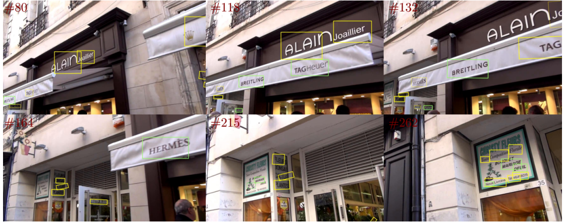
Figure 1.4: Output of the TextSpotter software for text localization and recognition. First, text is detected at some point in the video sequence (green regions) and then the region is tracked using the FoT tracker (yellow regions). The text detections are sparse and the FoT provides the text positions through frames where the detections are missing. Images courtesy of Michal Busta.
