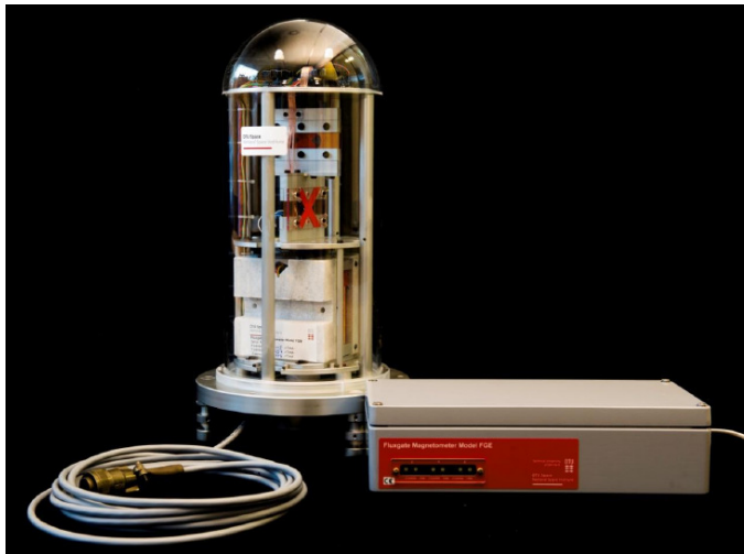
Figure 3.3: Magnetometer sensor with data logger [12]
