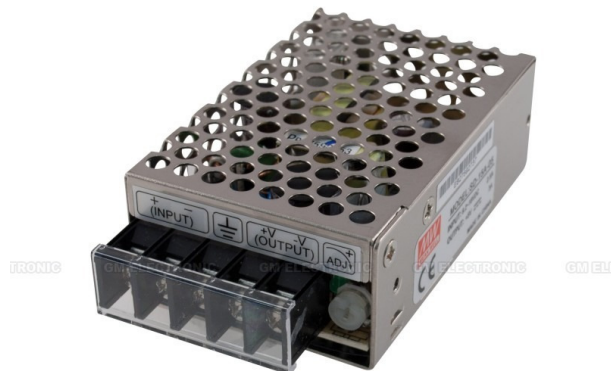
Figure 2.5: Photo of DC/DC converter Mean Well SD-15A-5 [10]
