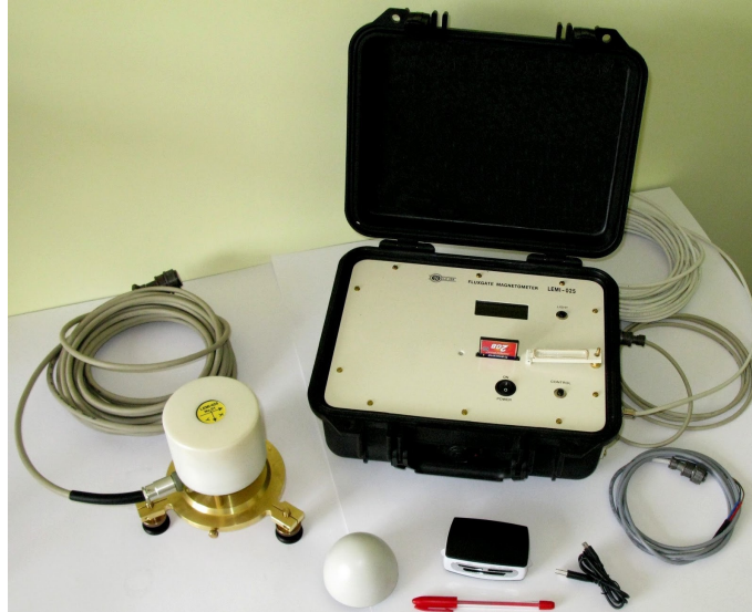
Figure 3.4: Data recorder for 3-component 1-second observatory Magnetometer LEMI-025 [14]
