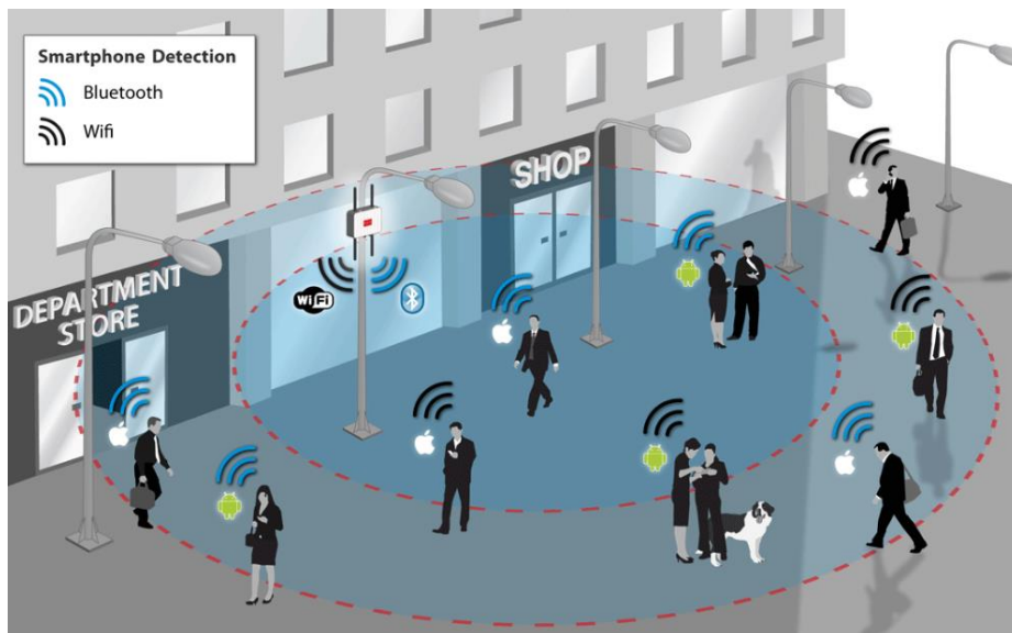
Figure 3-10. The Situation of hybrid indoor positioning system [3]
