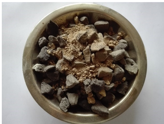
Obr. 6.19 Zemina smíchaná s Refaglass 8/16
